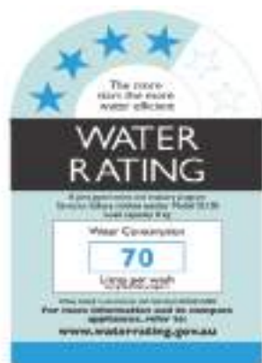
Figure 16: An Example Of The Water Rating Label Using As/Nz Standards
