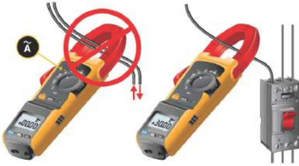
Figure 17: The Correct Way To Measure Current Using A Clamp Meter
